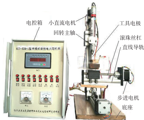
图1 微细电火花加工机床 Fig.1 Tool of micro EDM
